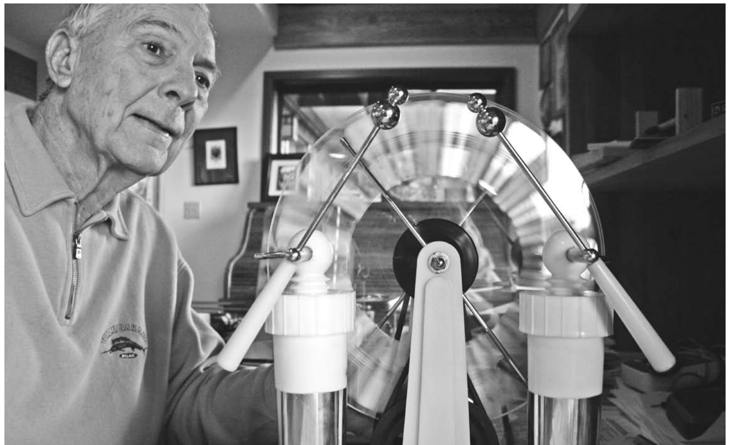
Paul Phelps demonstrates how a ham radio works with a spark gap. When enough charge builds, an electromagnetic wave will jump the gap, much like a radio wave shooting between a transmitter and receiver. Photo by Justin Nobel.
